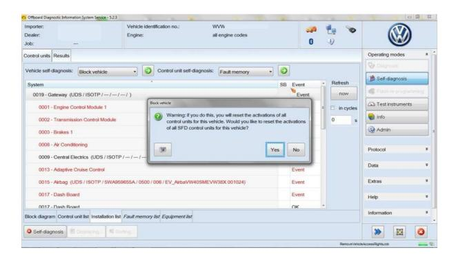
You will receive a response as to which control units have successfully been locked:
